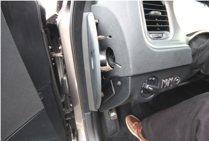
Removal of side panel; pulls off.
