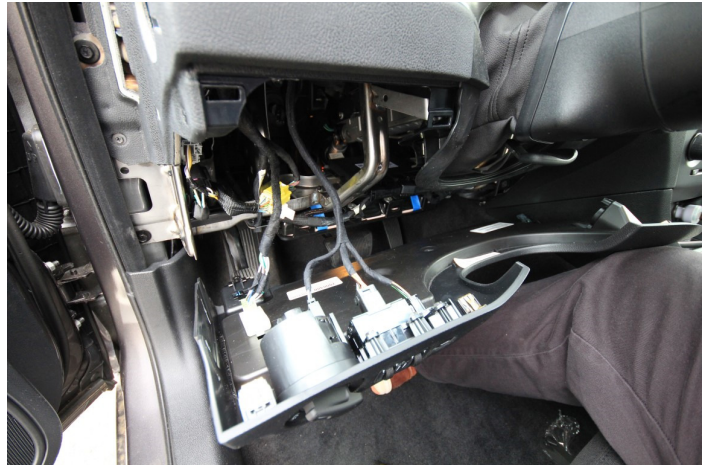
Remove 2 screws; pull lower cover straight back.
