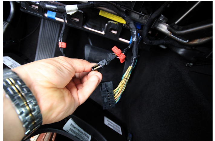
Right connector shown with 2 pin subconnector separated
