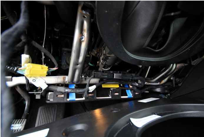
TCM located under steering column.
