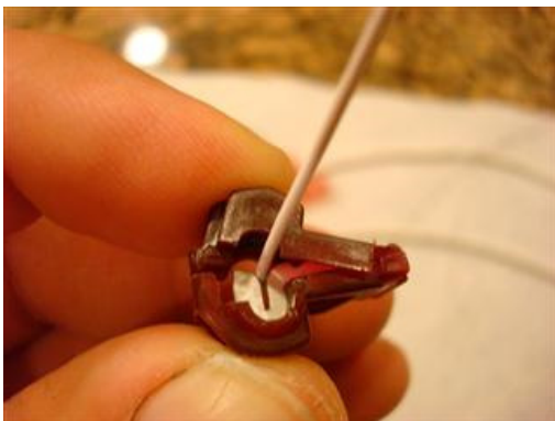
Correct application of t-tap on wire to be tapped.
