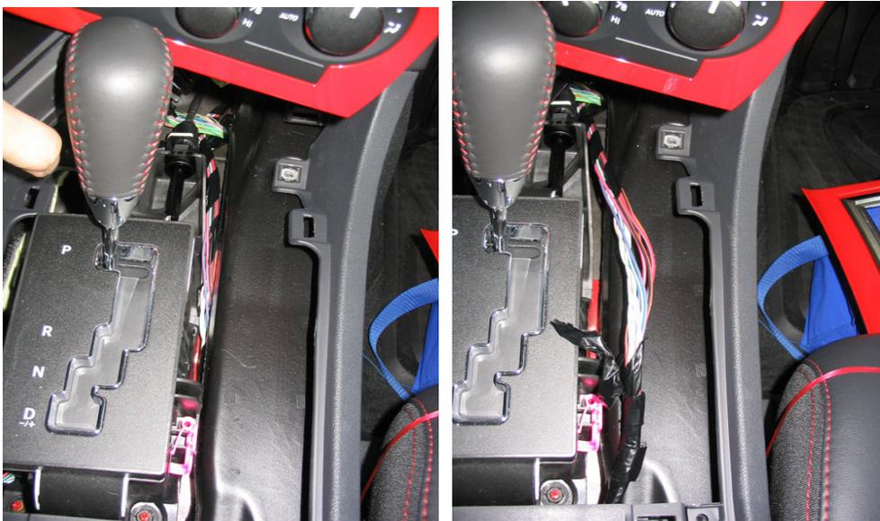
**Step 6:** Using the 3M wire taps provided, tap into the following wires that are in the harness that leads to the ESP button: Ground (black) from the NO-ESP board taps into the (black/light green stripe) wire. The ESP (green) wire taps into the (dark green/white stripe) wire.
