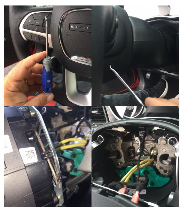
The airbag assembly disengaged and out of the way:
