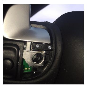
Once that's out of the way, there's one T20 Torx screw behind it, and one on the front of the switch assembly behind the airbag:
