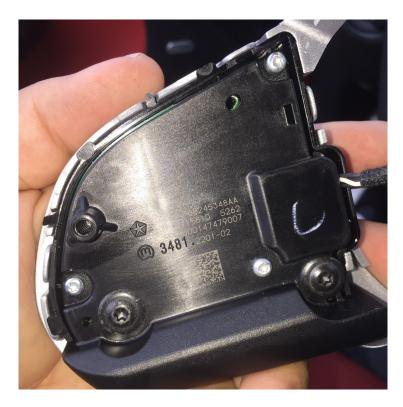
Assembly is basically the reverse. Plug the new switch back into the harness. Be sure to route the wires above the post that holds the front screw, so it's not behind the airbag. Replace the two T20 screws that hold the switch assembly in place. Replace the paddle shift switch, using its T20 screw and plastic cover. Push the airbag assembly back into place, it will snap back on easily. Lastly, re-connect the battery ground cable.
