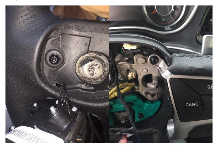
Remove those two screws, then unplug the switch assembly from the steering harness.
