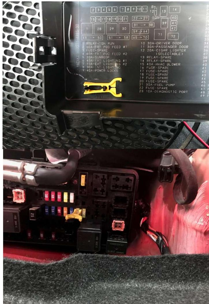
The add-a-circuit fuse tap will come with a 5A fuse already installed in the upper position. Plug the fuse you pulled from location 37 into the lower position (photo below shows it not installed)
