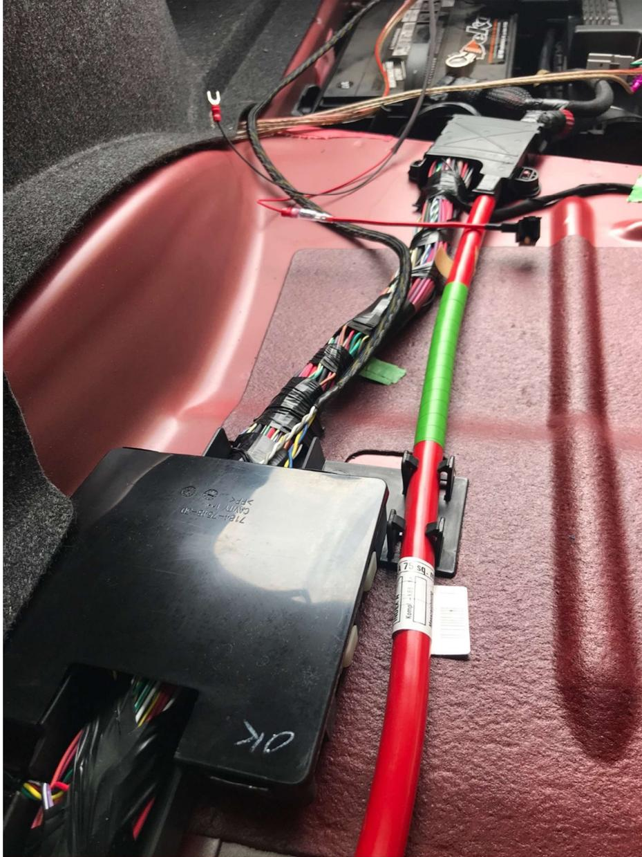
Lift off the cover of the fuse box behind the battery. In the cover, you will find a yellow tool that is used to remove fuses. Locate and remove fuse 37.
