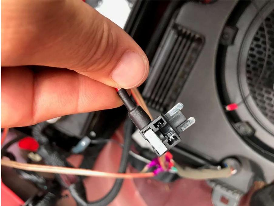
Plug the add-a-circuit into the slot for fuse 37 as shown.
