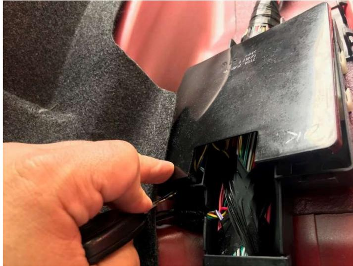
Plug the blue plug of the Double Bypass harness into the WHITE STAR connector that has the green plugs. Plug the black plug into the GREEN STAR connector that has white plugs. Any available slot will work.
