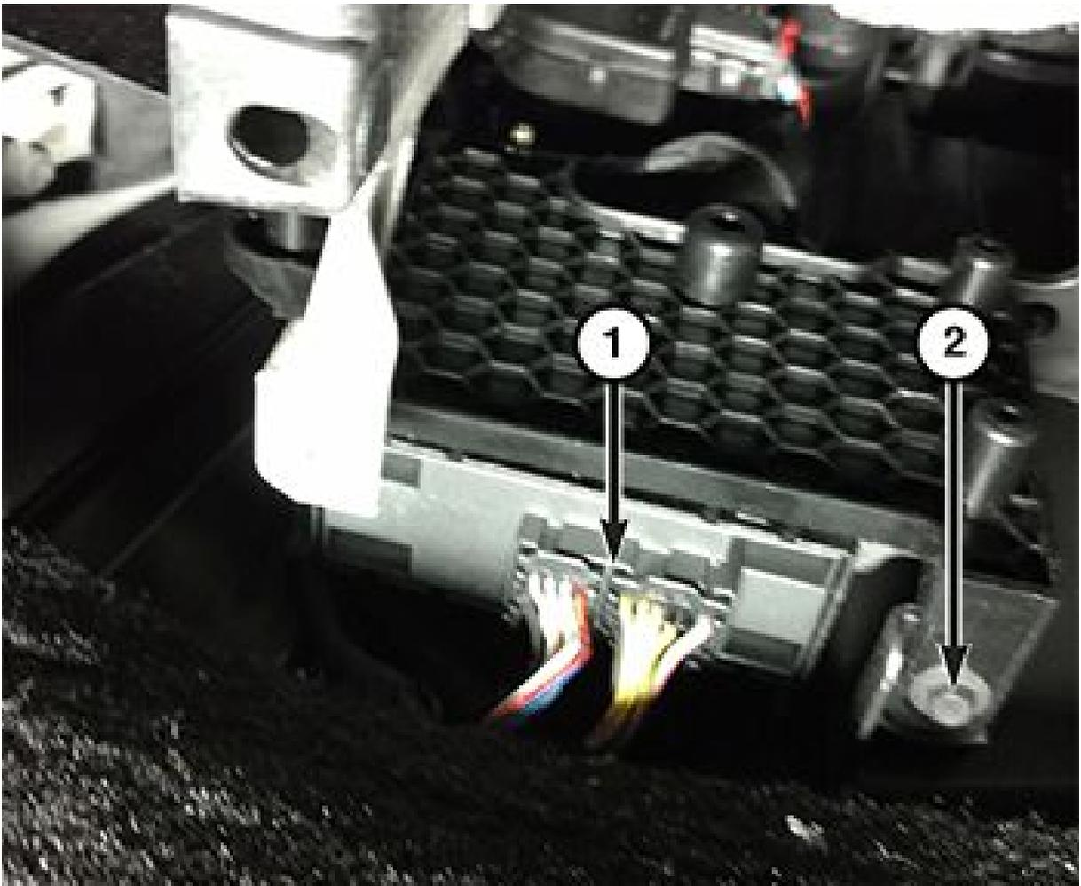
Step 3: Plug in Security Bypass Block into Existing Connectors and tuck up inside. Reinstall Push pins holding silencer panel in place.
