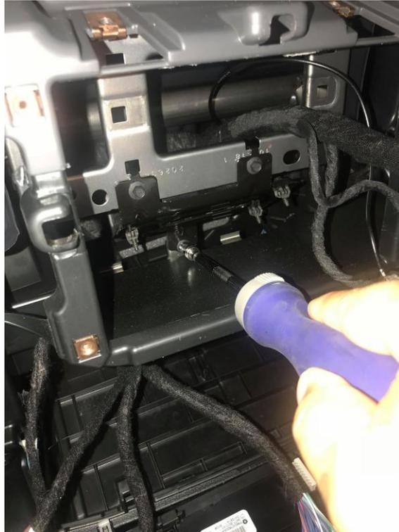
**Step 7: Unplug connectors going into Security Gateway Module (1)**
