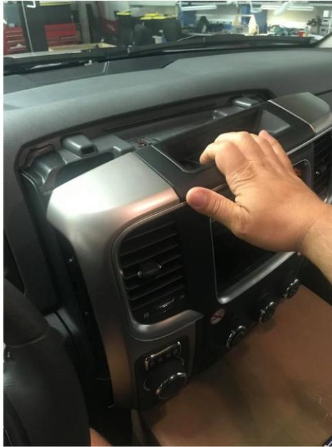
**Step 4: Remove the four fasteners securing the Radio to the instrument panel**
