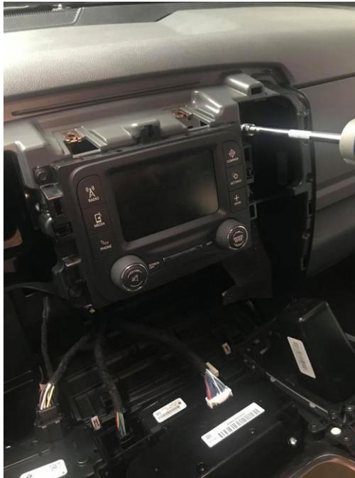
**Step 5: Remove the radio from the instrument panel.**
