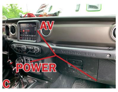
Route the inside portion of the cable behind the glove box through the passenger side grommet. (A, B)
