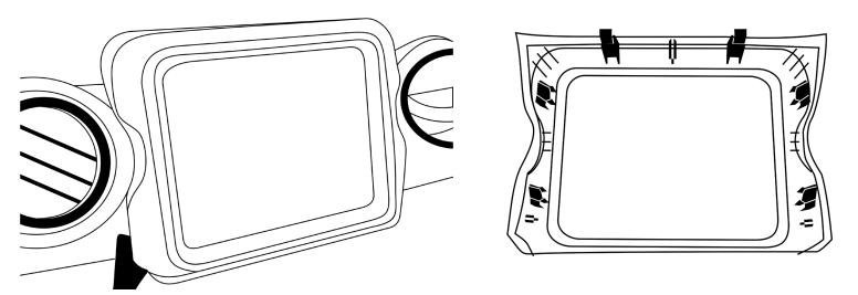
Once screws are removed, use a trim stick to remove bezel from dash.
