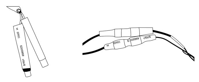
Place the included shrink tubing over one side of the camera connectors, then plug in the mating connector, making sure to cover both connectors with the heat shrink. Center the heat shrink, then use a lighter or heat gun to constrict the tubing over the connectors.
