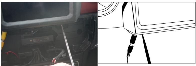
Using a Phillips head screwdriver, remove two screws holding radio bezel to dash.
