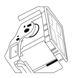
Using a small flat head screwdriver, raise red terminal locking plate off the main radio connector.
