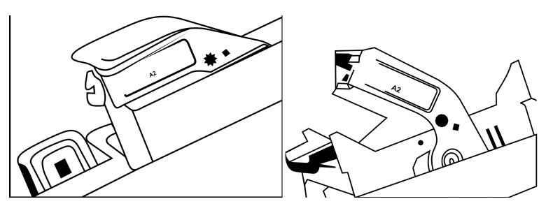
Unlatch the large radio connector arm and raise the arm to release the connector.
