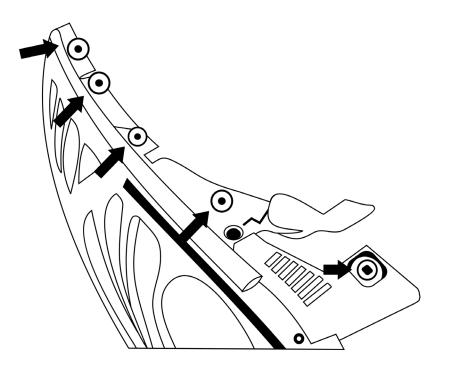
Remove the 5 clips holding the top of the grille to the core support. Once removed, you can lean the grille forward to aid in installation.
