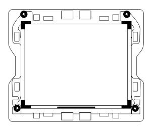
Using a phillips head screwdriver remove the 4 screws holding the radio into the dash.
