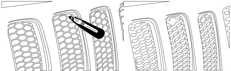
Using a box cutter or wire snips, trim middle grill slating to fit camera bracket.
