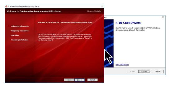
Accept the default and click Next. Allow the FTDI driver package to install too. Once installed, the ZPU icon will appear on your desktop and in the App list under "Z Automotive"
