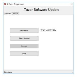
**Manual Update**: Clicking the Manual tab will switch the updater to manual mode. This allows you to load in any firmware supported – which can be an older version from the Z Automotive website, an experimental beta version, or one emailed to you from customer support.
